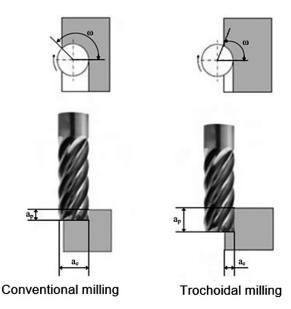
**Fig. 1.** Comparison of the idea of conventional and trochoidal milling, where:  $a_p - milling depth$ ,  $a_e - width of cut$ ,  $\omega - tool arc of engagement [6]$
