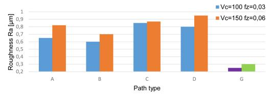
Fig. 4. Influence of path type on roughness parameter Ra of grooves walls
