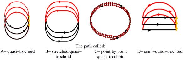
Fig. 3. Paths used in trochoidal milling
