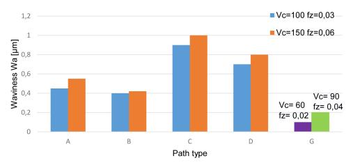
Fig. 5. Influence of path type on waviness parameter Wa of grooves walls
