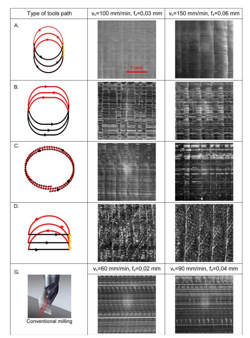
Fig. 6. Photos of groove walls with variable machining parameters and various trochoidal tool paths
