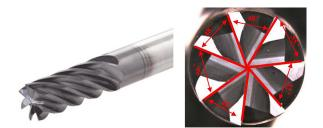
**Fig. 2.** Iscar milling tool – 7– flutes with different helix and variable pitch for trochoidal milling
